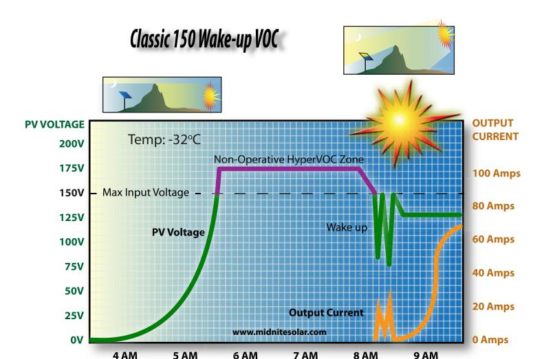
On cold mornings the PV panels will put out full voltage even before you can see the sun. Ambient light may not have much current behind it but it does have voltage exceeding the possible voltage limits that destroy the controller. The fact that there is no power behind the output voltage means that the controller will not be able to turn on and drag the panels down from VOC to max power voltage.
